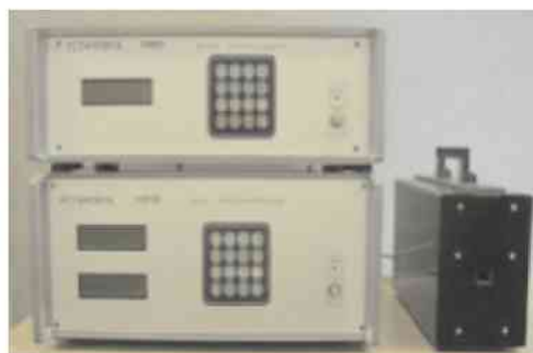
INSTALLATION FOR MEASUREMENT OF CHANGES OF MAGNET FERROMAGNETIC CHARACTERISTICS IN QUASI-STEADY MODE
