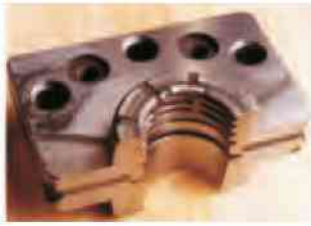
2. Forms of casting of gas-burner and neck of bottle after laser surfacing
